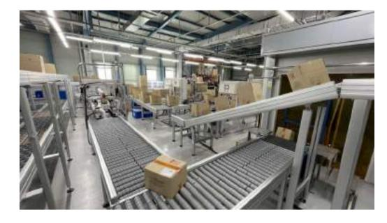
Pre-programmed flat BLDC Gear Motors are built into the frames for a smooth installation process. All Avancon's conveyors are built as standard zones, which automatically results in 'Zero Pressure accumulation' (ZPA) at any position even on slopes, and which also saves energy for the entire system and reduce cost.
