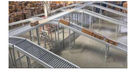
**Sorter**: The Avancon OTU- sorter smoothly moves goods — exchange parts for motor cicles and bicycles in a curved path to the right or left, making sorting and distribution more efficient.
