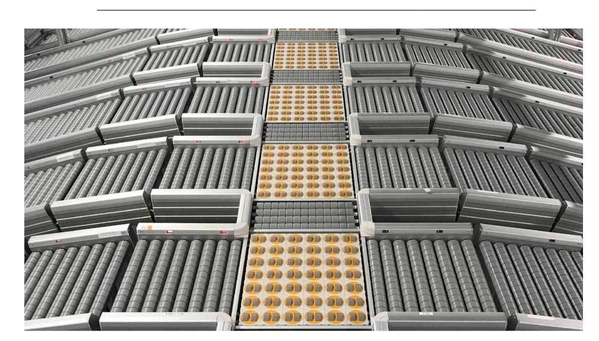
The Avancon-OTU is a versatile unit that can move all goods with a flat base in any direction. It fits into nearly all conveyor setups using special aluminum frames and comes fully assembled with motors and controls tailored for your needs.
