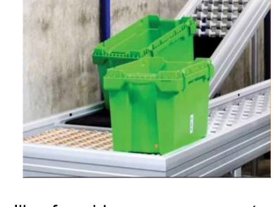
The OTU tables can be used in many other situations, like for sideways movements before barcode readers, in high bay storage picking, moving goods around corners, or taking items off a powered line for inspection.
