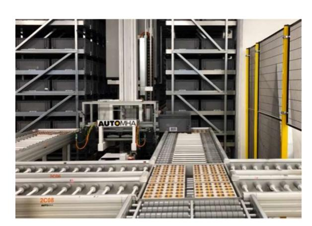
Because the Avancon roller- and belt-conveyors are designed to work in zones and are already set up to communicate with each other, there's no need for an external control cabinet, control box, or anything like that. This makes it easy and economical for any machine manufacturer to use and offer the machine-concatenation or production line as a full package composed of their machines and the required conveyors to their customers.
